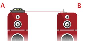
5. USE ADJUSTMENT TOOL TO TURN FINIAL DOMES UNTIL LASER BEAM MATCHES UP WITH CROSSHAIRS ON TARGET ON SPEAKER 'B'
